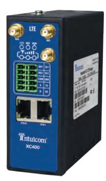
Intuicom's XC400™ is a feature-rich industrial router that delivers LTE connectivity demanded in mission critical applications. Designed to provide the crucial link to your remote devices and provide Industrial Internet of Things (IIoT) connectivity, the XC400 provides secure, robust communications across a broad variety of equipment and applications.
