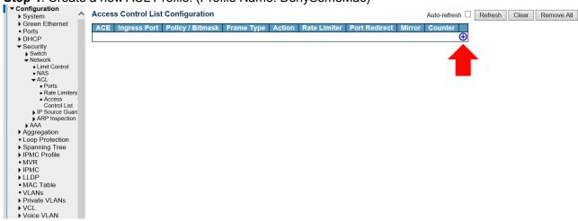
Step 2: Create a new ACL Entry rule under this ACL profile. (Deny MAC: 11 and VLAN: 4)
