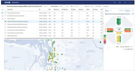
Signal Analytics display of intersections in Austin, TX. Each intersection can be selected to reveal detailed metrics at the movement level.
